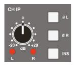
The X-Panda Stereo Input channels (**CH IP**) feature a +/- 20 dB gain stereo **Level Trim**, indented in the centre at Unity Gain and a pair of independent Phase Reverse "**Ø**" switch for both the L+R Inputs.
